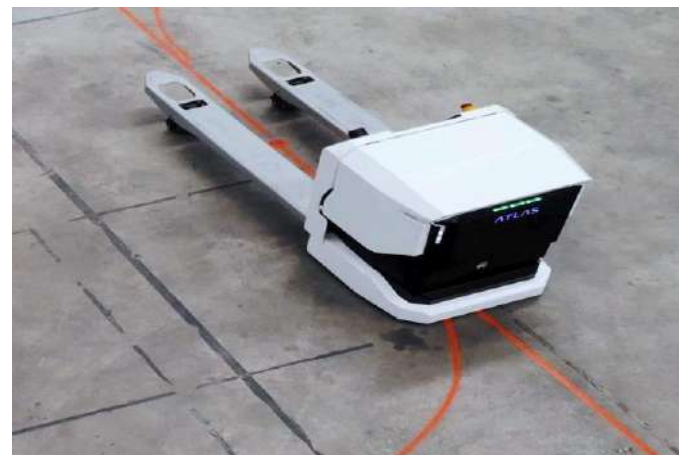
ROBOT AUTONOMOAK AGV Automated Guided Vehicles
